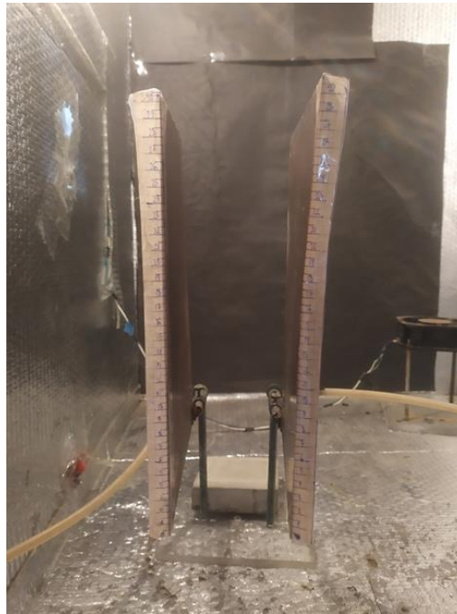
Fig.4. Condenser plate system
