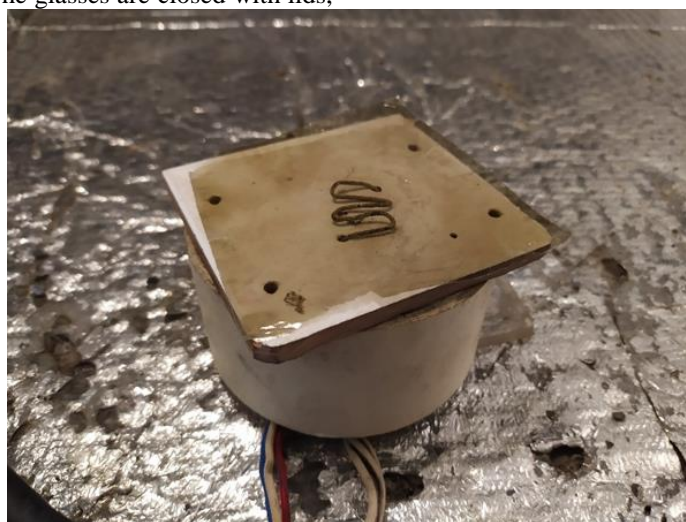
Fig.3. Reagent sublimation device
